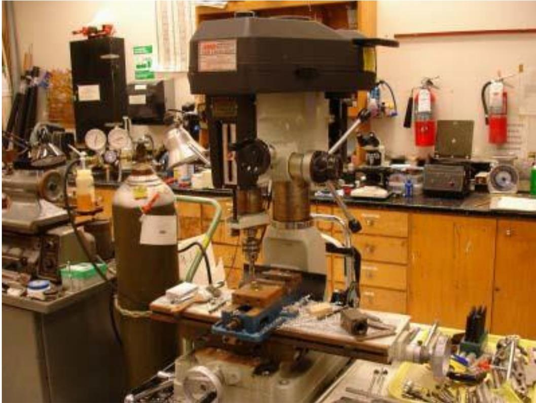
The Maintenance Shop also has: a drill press for drilling general purpose holes up to 1" in diameter in metal and 3" to 4" holes in plastic or wood; a horizontal metal saw for cutting metal and plastic bars, and rods up to 4" in diameter; a chop saw for end cuts on wood or plastic up to the size of a 2" x 4"; and a bench vise.
